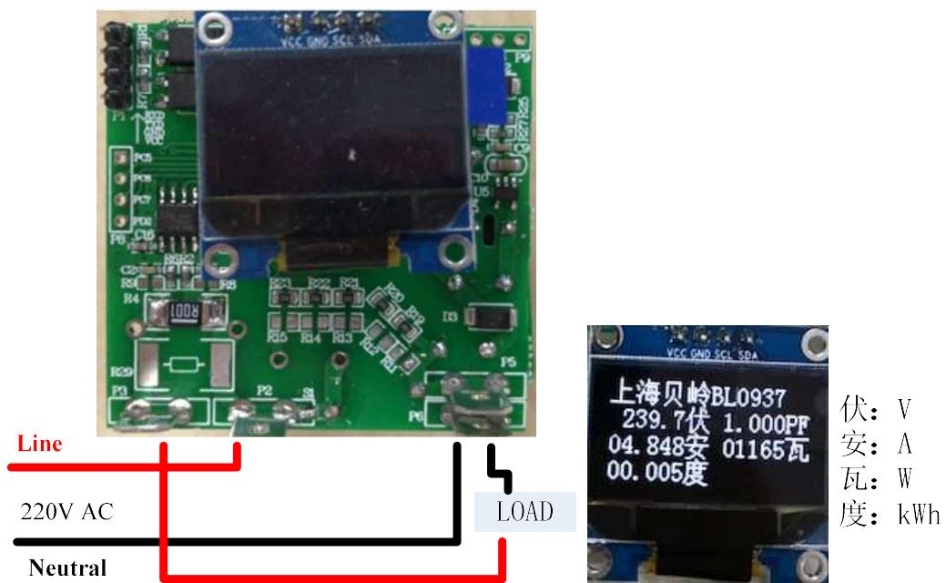
The schematic of the BL0937 evaluation board:
